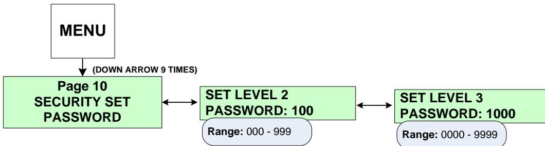
**SP10.1 Set Level 2 Password:** This level uses a 3-digit password. The default level 2 password is 100.
