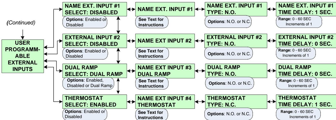
**SP6.5 User Programmable External Inputs:** The controller provides up to 4 digital external inputs which are individually programmable. A description name can be assigned to each individual input for easy identification.
