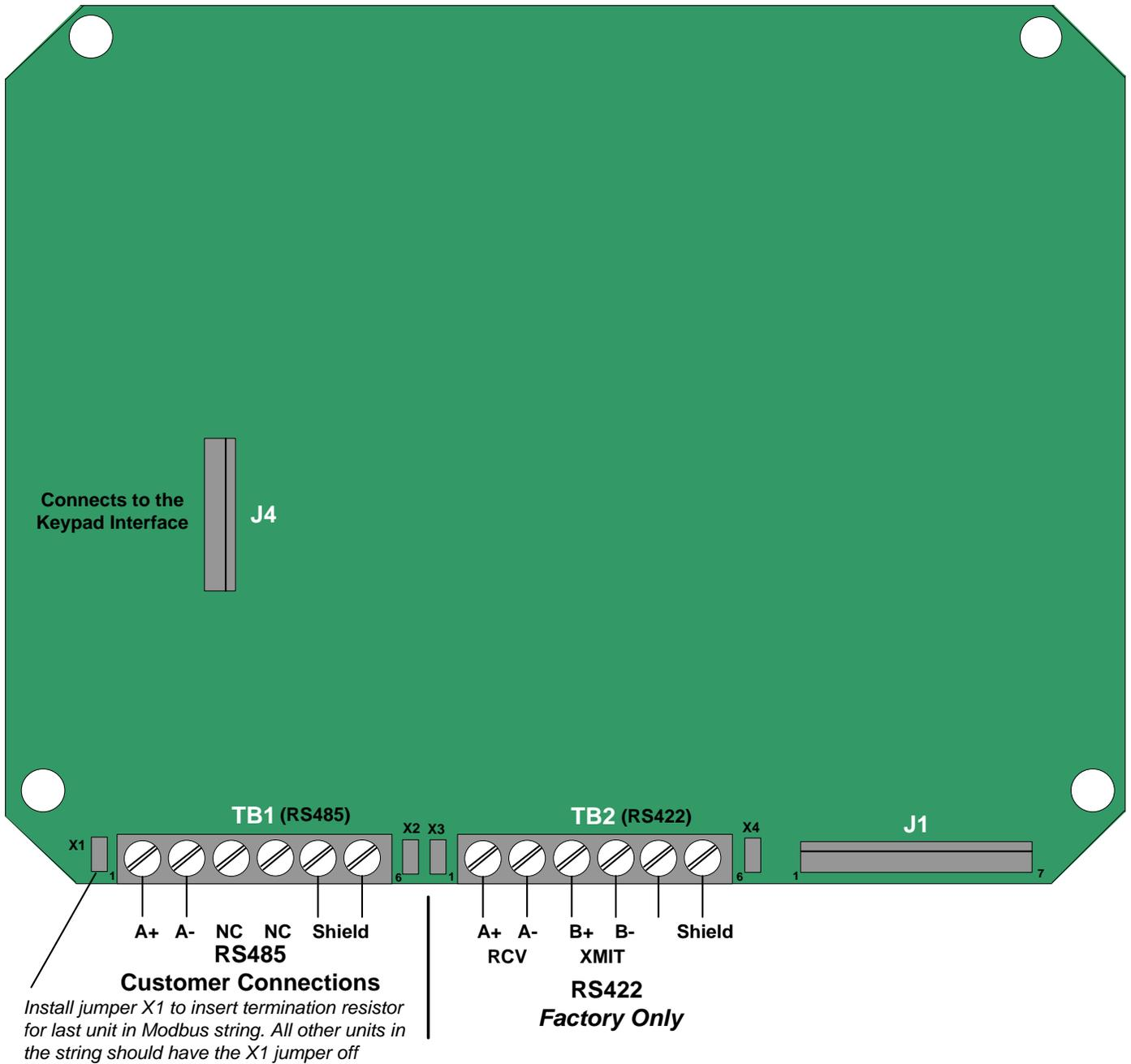
FIG. 2.9d RS485 / RS422 Communications Board
