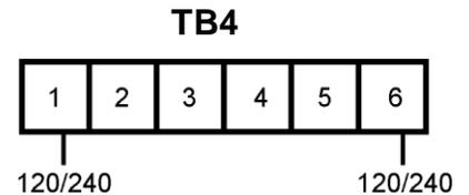
Unit comes standard with 120VAC control. Order 240VAC control as an option if required.
