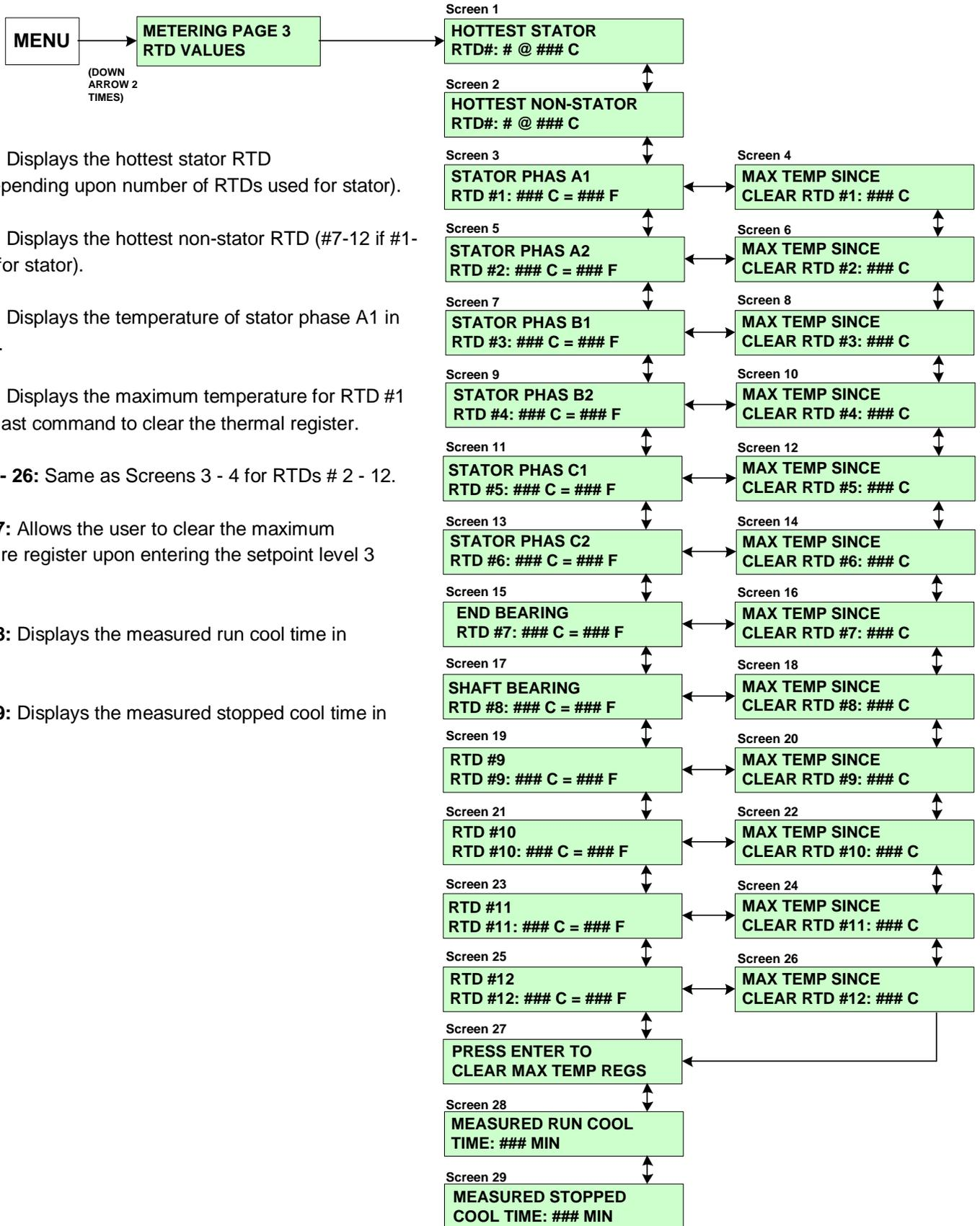
**Screen 1:** Displays the hottest stator RTD (#1 – 6 depending upon number of RTDs used for stator).
