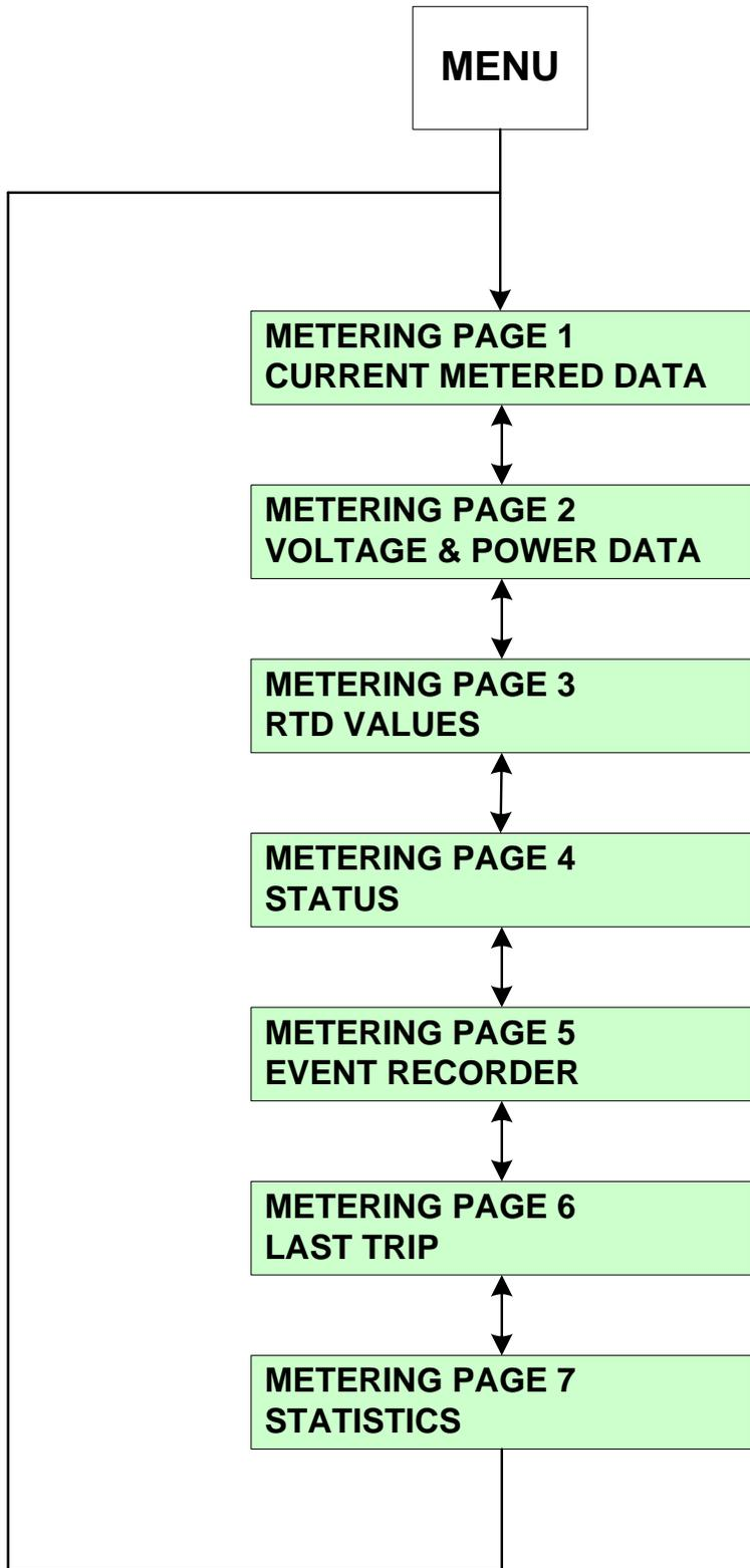
**MP.1 Metering (Metering Page 1):** Displays basic current metering data.
